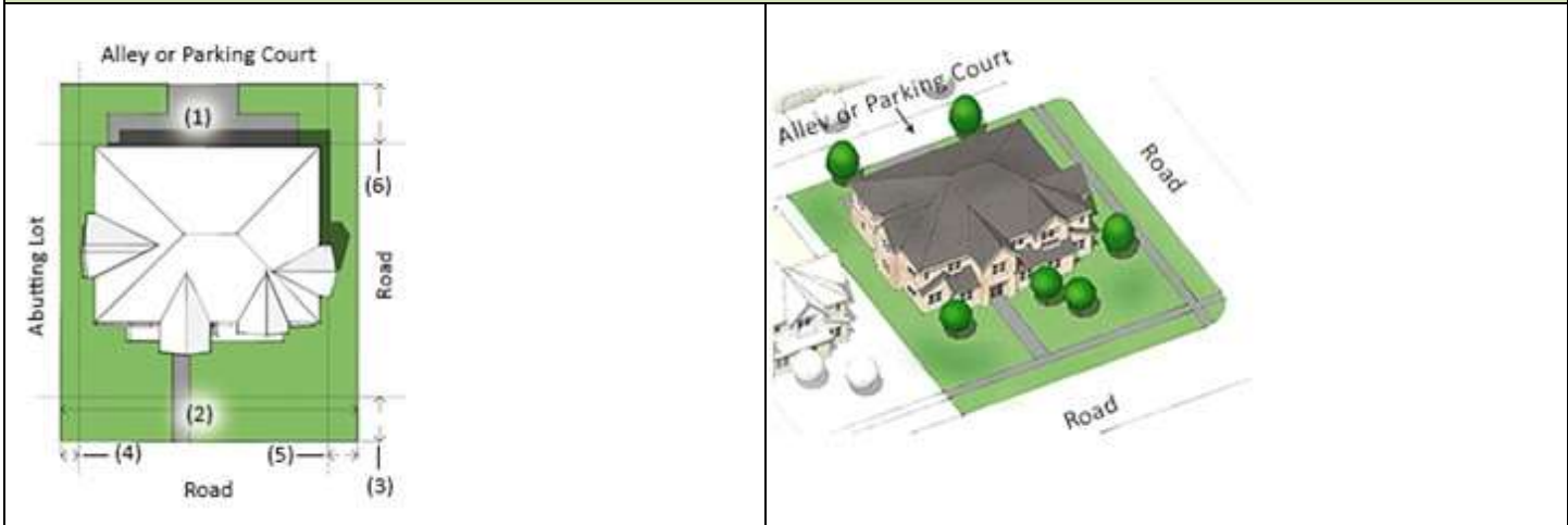
Legend: 1. Minimum lot area; 2. Minimum lot width; 3. Front yard; 4. Interior side yard; 5. Street side yard; and 6 Rear yard.
