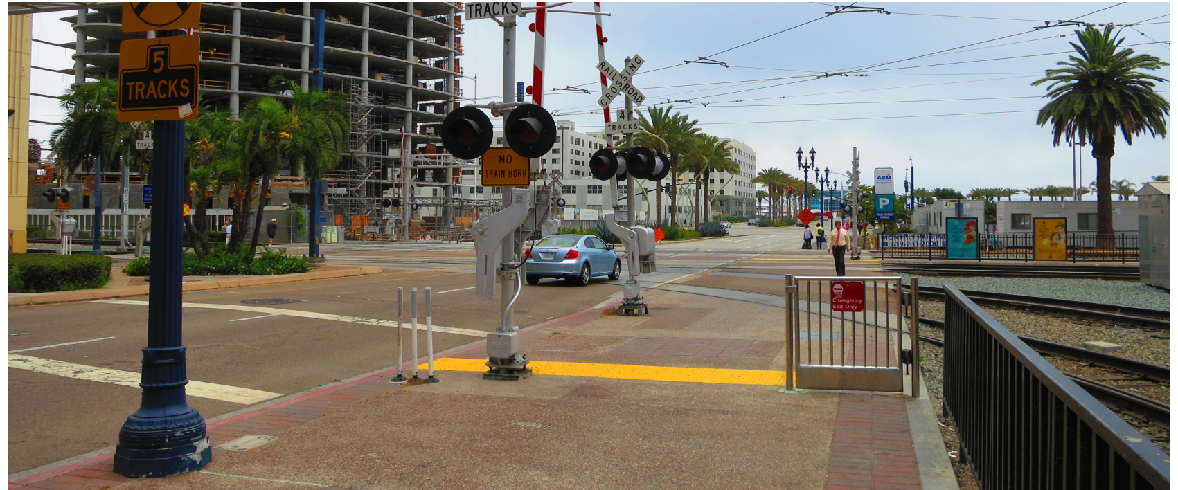
Example pedestrian facilities at railroad crossing in San Diego, California
