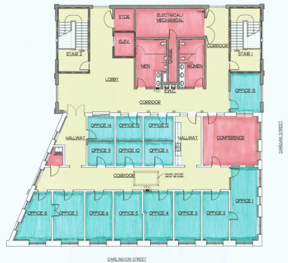
RENOVATED SECOND FLOOR PLAN NORTH SCALE: 1/8" = 1'-0"
