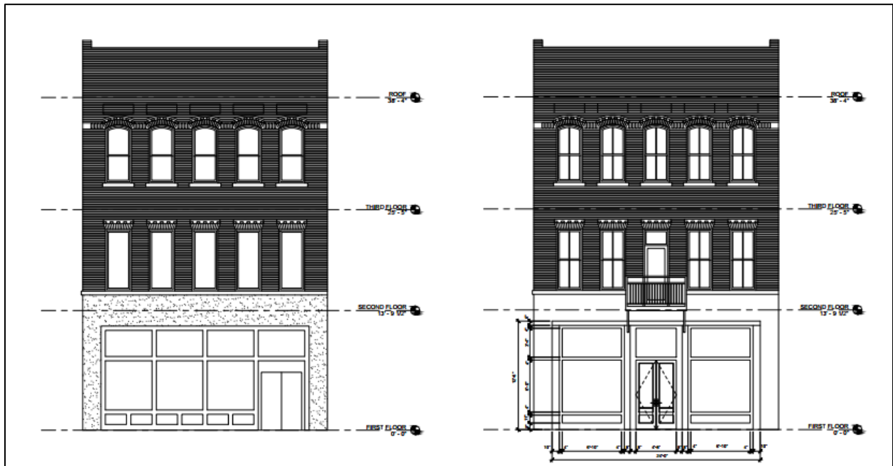
South elevation (front of building): existing on the left; proposed on the right.
